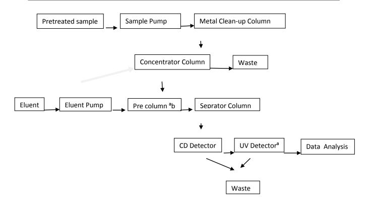
Fig;4.1 Schematic representation of an ion chromatography system, including online preconcentration system
